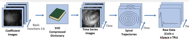
**Figure 4.** Forward model of the dictionary constrained reconstruction
