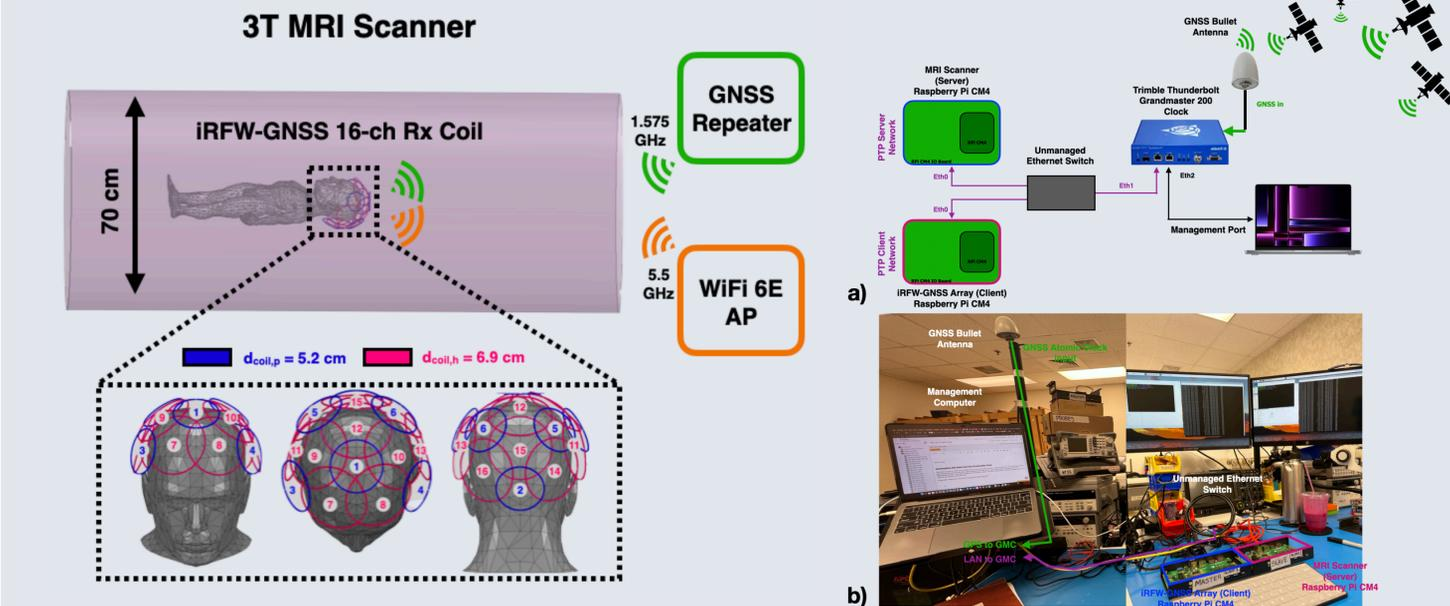
**FIGURE 2. Simulation Model** 16-channel coil soccer-ball array with six 5.2 cm diameter (blue) and ten 6.9 cm diameter (pink) coil elements simulations were performed inside a 70 cm scanner bore at the 3T Larmor (127.7 MHz), WiFi 6E (5.5 GHz), and GNSS (1.575 GHz) frequencies to determine its MRI SNR and WiFi 6E/GNSS far-field gain patterns producing the most radiated signal outside the scanner bore to an access point (AP) or GNSS repeater on scanner room wall.
