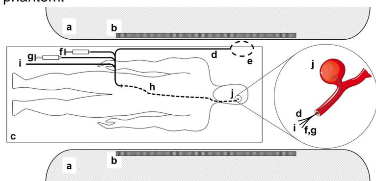
**Figure 1:** MRC concept. (a) MRI scanner magnet assembly. (b) Body RF coil. (c) Patient table. (d) Long wire RF pickup antenna magnetically coupled to body coil; RF pickup may be optionally enhanced with tuned RF pickup loop (e) connected to free end of wire. (f) Protein solution and (g) saline for flushing sharing one lumen of catheter (h) inserted percutaneously into femoral aorta. (i) Fiber optic temperature sensor sharing second lumen of catheter with wire. (j) Cerebral aneurysm.
